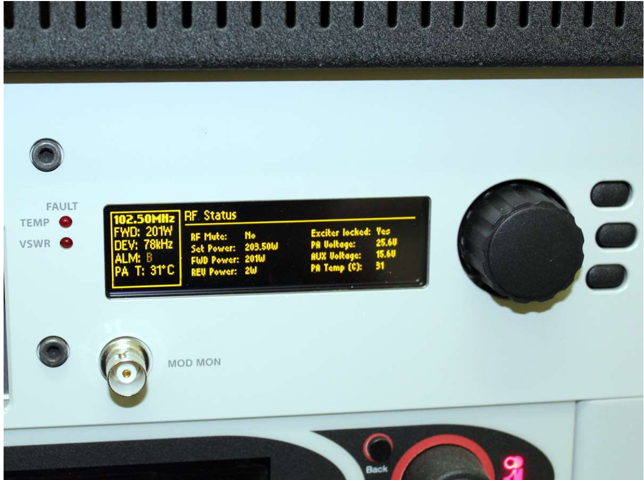
Picture of transmitter showing operating power level of 201 Watts.
