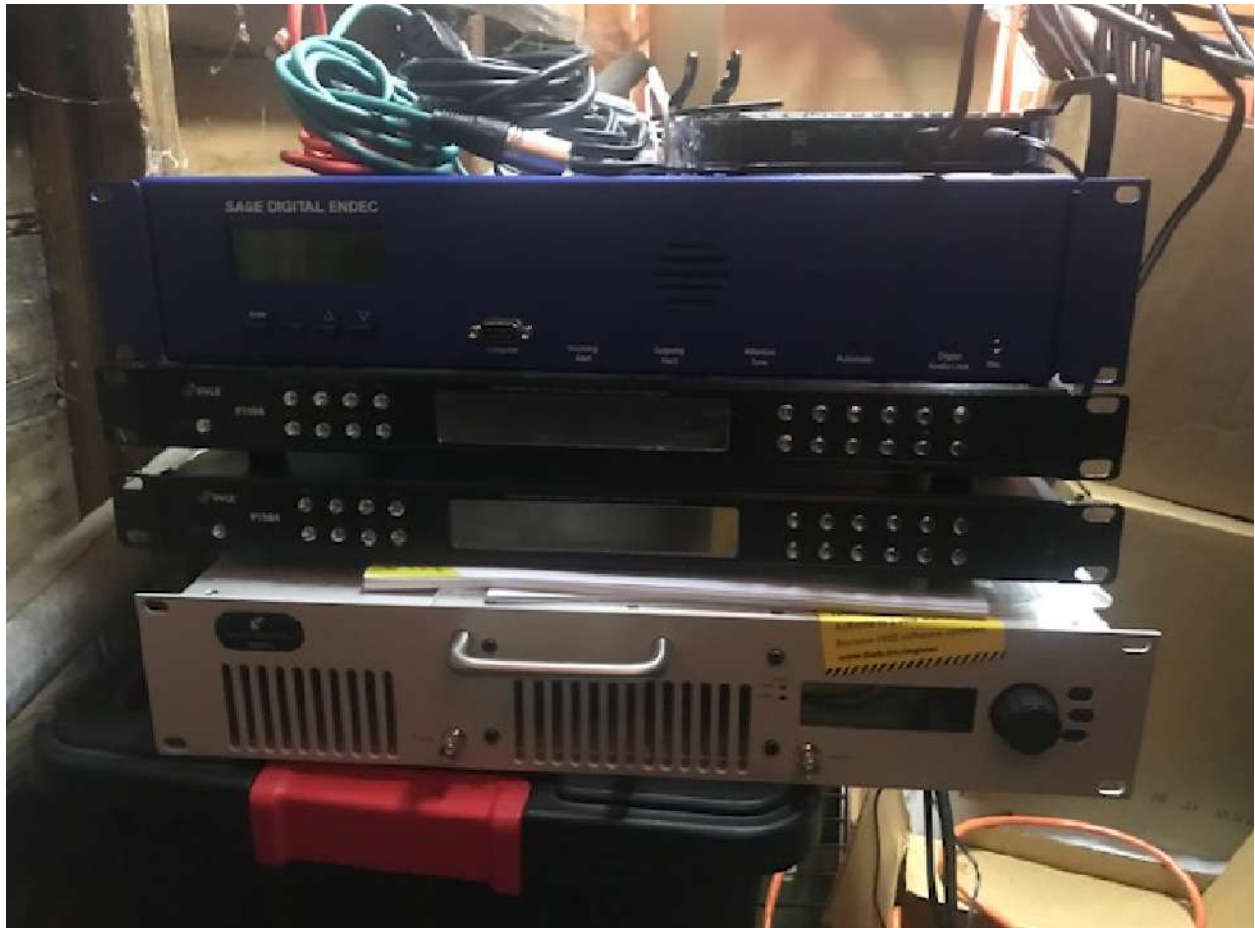
Equipment being used (BW Broadcast transmitter, Sage Endec) (photo taken in Futrell's garage at first construction date)
