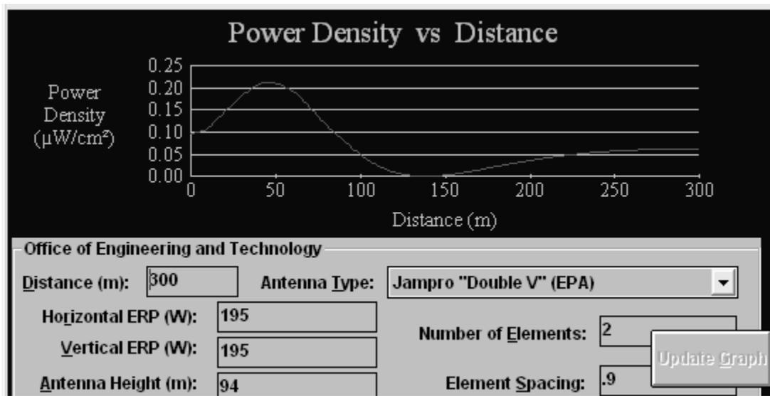
The Max Power Density was found to be .212851267556061  $\mu\text{W}/\text{cm}^2$  at 44 meters.
