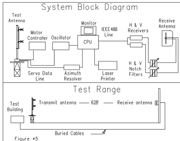
The antenna under test was operated in the transmitting mode and fed from a HP8657D signal generator. The frequency of the signal source was set at 89.3 MHz and was constantly monitored by a Rohde & Schwarz ESVD measuring receiver.
