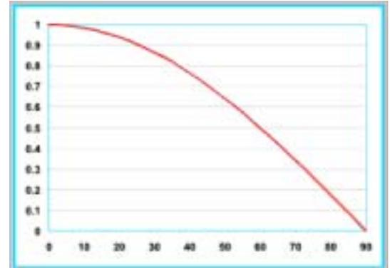
VERTICAL PATTERN PLOT of SHIVELY model 6813 ==> 2 Bay FM Broadcast Antenna in use at KWWV(FM)
