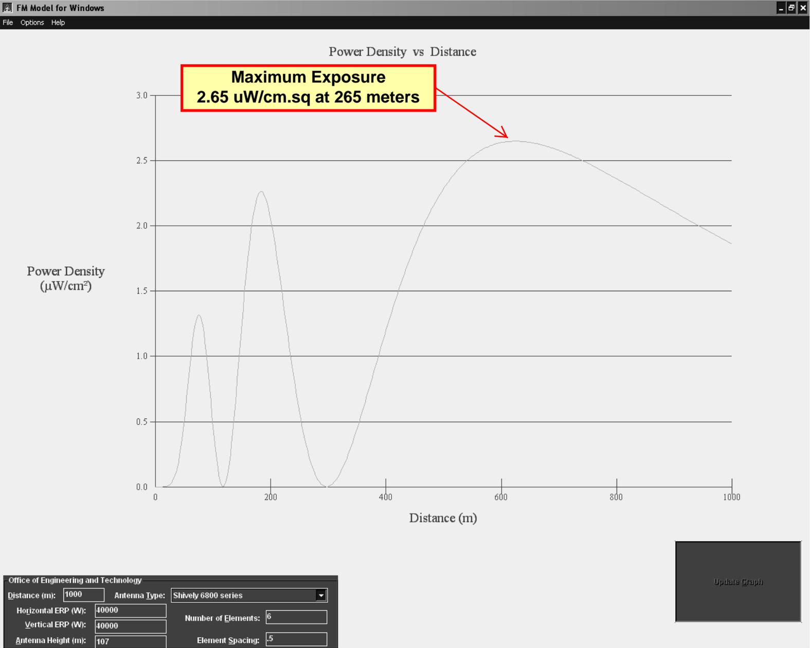
WLOB-FM operates with a Shively 6810-6R-SS-DA with a bay to bay spacing of 0.5 lambda with the center of radiation at 107 m or 351 feet AGL.
