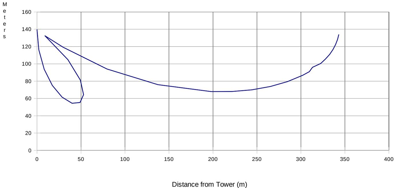
Location of 100.5 dbu contour above ground, versus distance from tower.
