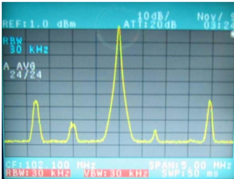
Digital image of the KMJQ auxiliary transmitter, indicates response 600kHz + from center carrier. Horizontal display grid is 300kHz per division/3Mhz Span. Vertical display grid is 10db per division. 30kHz bandwidth is used during measurements. Within the limits of the linearity of the analyzer, the skirts indicate sideband energy to be more than 70db below peak carrier at 600kHz.
