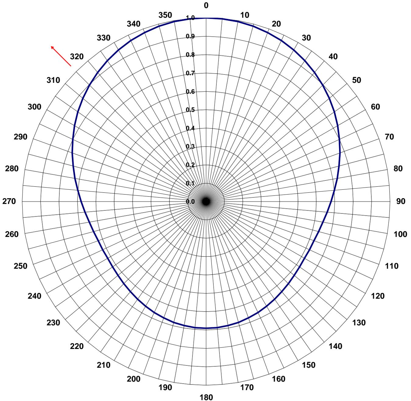
**TABULATED DATA FOR AZIMUTH PATTERN****TYPE: ATW-GS**
