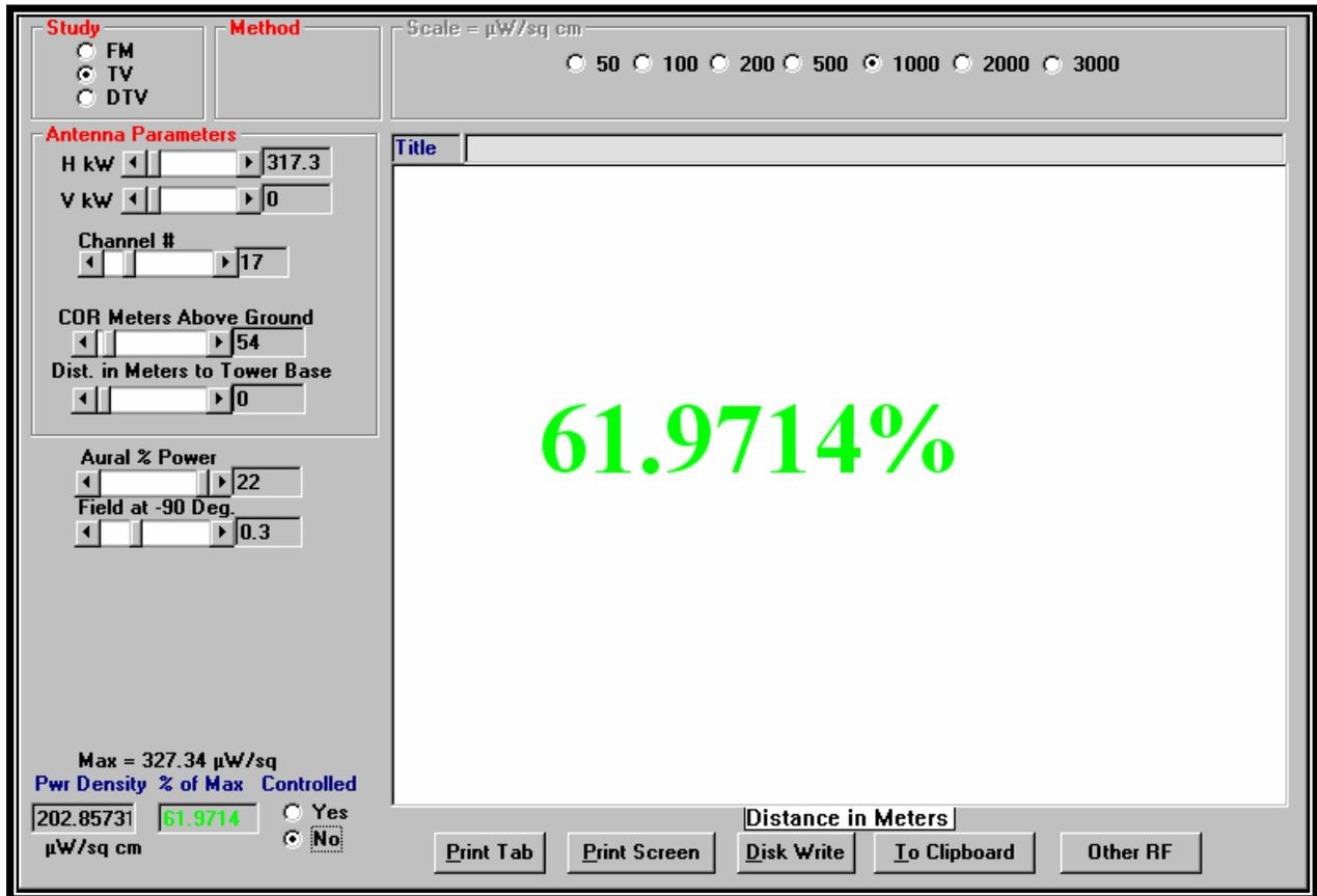
The “Dist to COR” value shown on the above graph represents the height of the antenna center of radiation above an observer on the ground who is assumed to be 2 meters in height.
