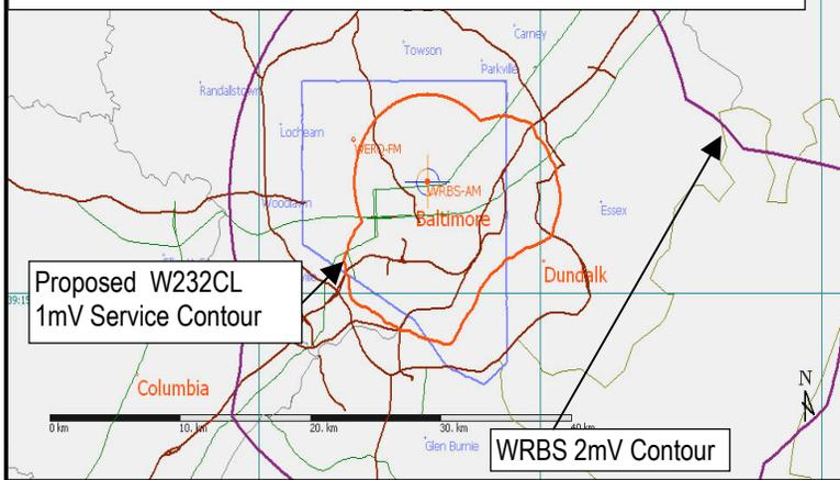
Note that the W232CL 1mV service contour extends less than 40km from the WRBS antenna site
