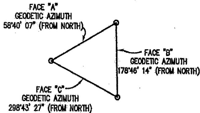
This Plat is to certify the Geodetic Azimuths of the sides of the Burk Road Tower that the ERI model 1083-5CP-DA directional antenna has been attached to. The tower is located at the southeast corner of Burk Road and Post Road in Indianapolis, Indiana. (address: 9301 East Burk Road). The Geodetic Azimuths are taken from Ellipsoid: GRS80/WGS 84 (NAD83).
