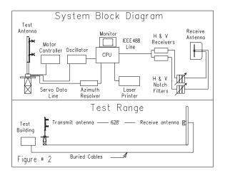
position indicator. The resolution of this angle position indicator is one-hundredth of a degree.
