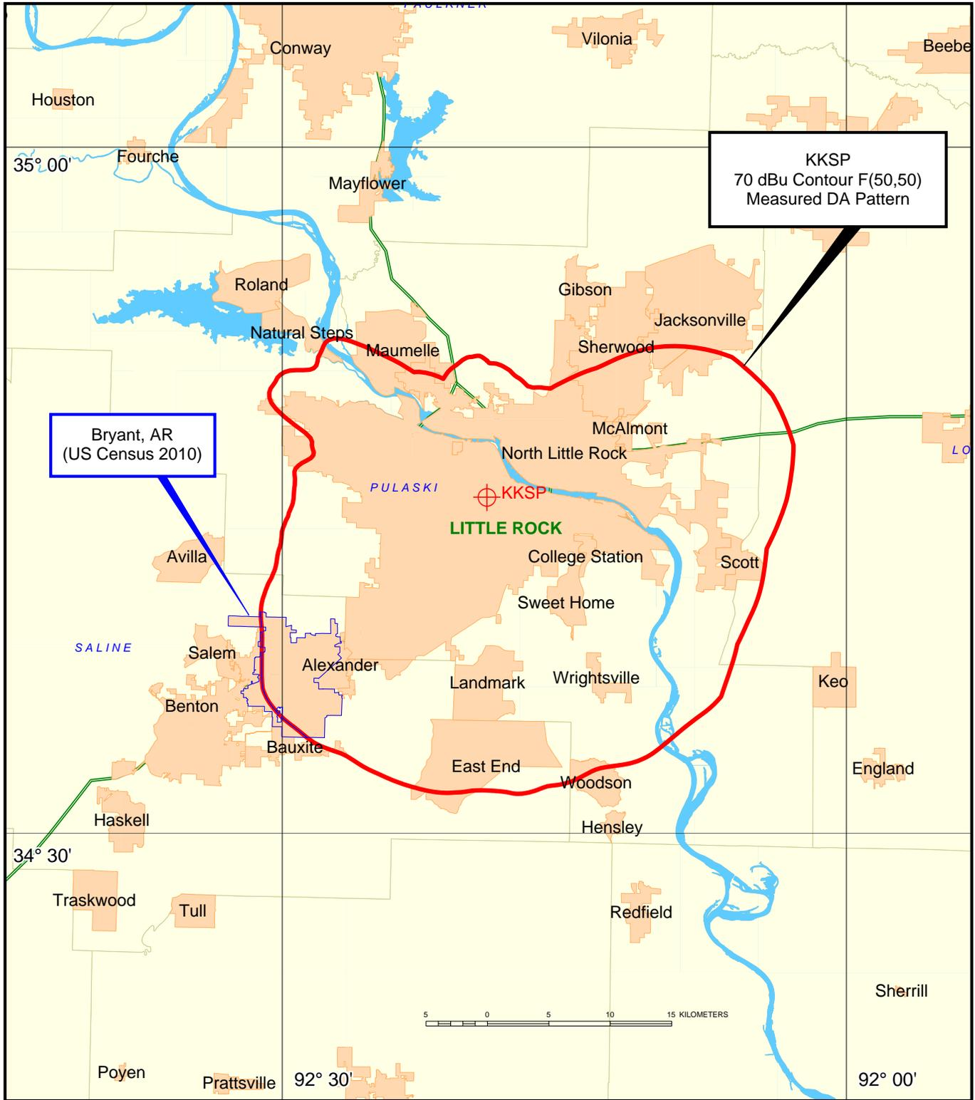
**SECTION 73.315 STUDY BASED ON MEASURED DIRECTIONAL ANTENNA COMPOSITE AZIMUTH PATTERN KKSP(FM), BRYANT, ARKANSAS CH. 227C3, 22.0 kW (DA-MAX), 107 m HAAT JUNE, 2016**
