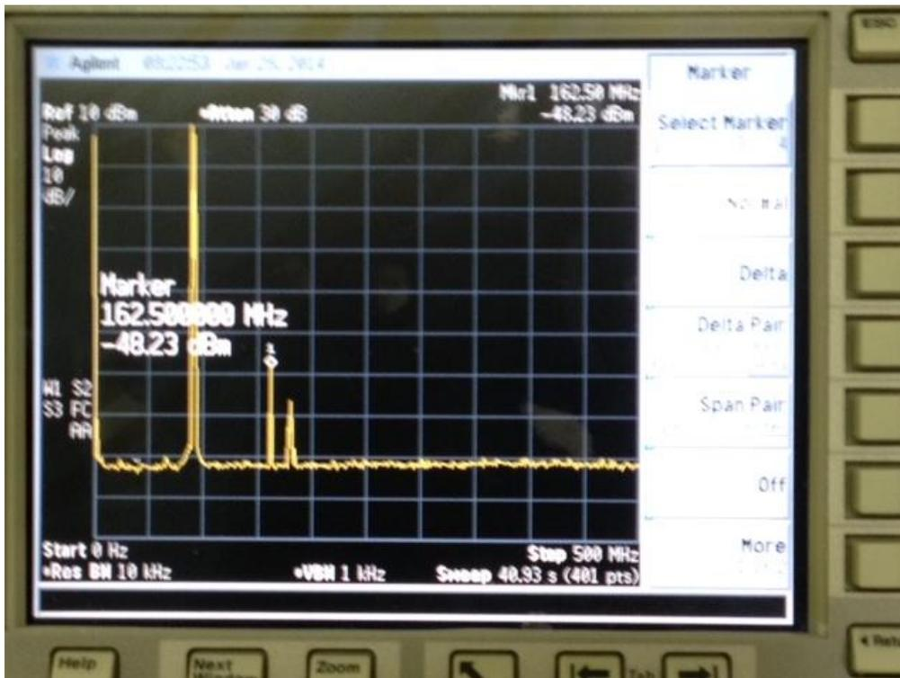
The image below was the result of the insertion of a tuned notch filter with an out-of-notch insertion loss of less than 1dB, and a 3dB bandwidth of approximately 3MHz. This filter reduced the amplitude of the fundamental signals on 89.7MHz and 91.9MHz sufficiently to eliminate the analyzer-induced spurious emissions, however the co-located NOAA weather transmitter signal remains, as indicated by the marker.
