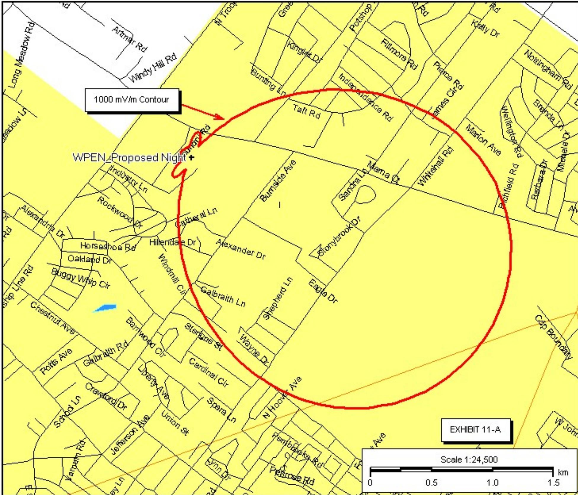
Computed Nighttime 1000 mV/m Contour For The Proposed 21 kW Nighttime Operation Of WPEN, Philadelphia, PA
