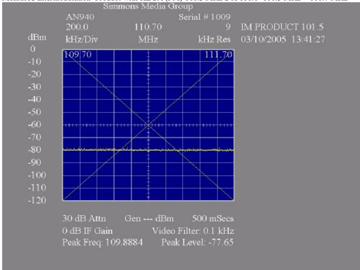
Measured Intermodulation Product with KJQN (FM) 103.1 MHz 2 X 106.1- 103.1 MHz = 109.1 MHz
