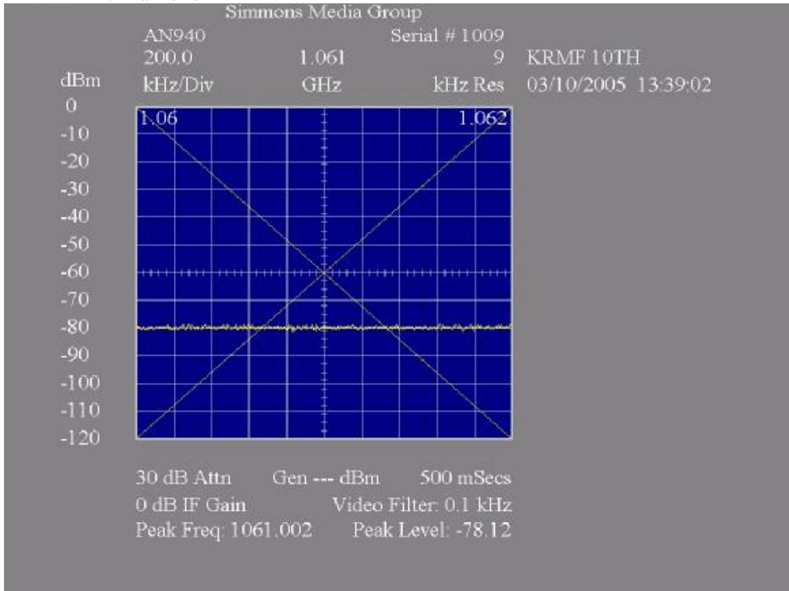
Measured Intermodulation Product with KEGA (FM) 101.5 MHz 2 X 106.1- 101.5 MHz = 110.7 MHz
