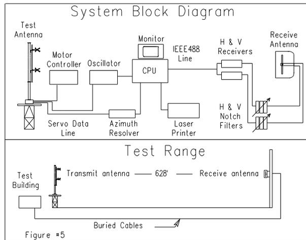
The antenna under test was operated in the transmitting mode and fed from a HP8657D signal generator. The frequency of the signal source was set at 91.5 MHz and was constantly monitored by a Rohde & Schwarz ESVD measuring receiver.
