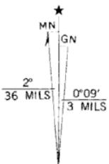
UTM GRID AND 1976 MAGNETIC NORTH DECLINATION AT CENTER OF SHEET
