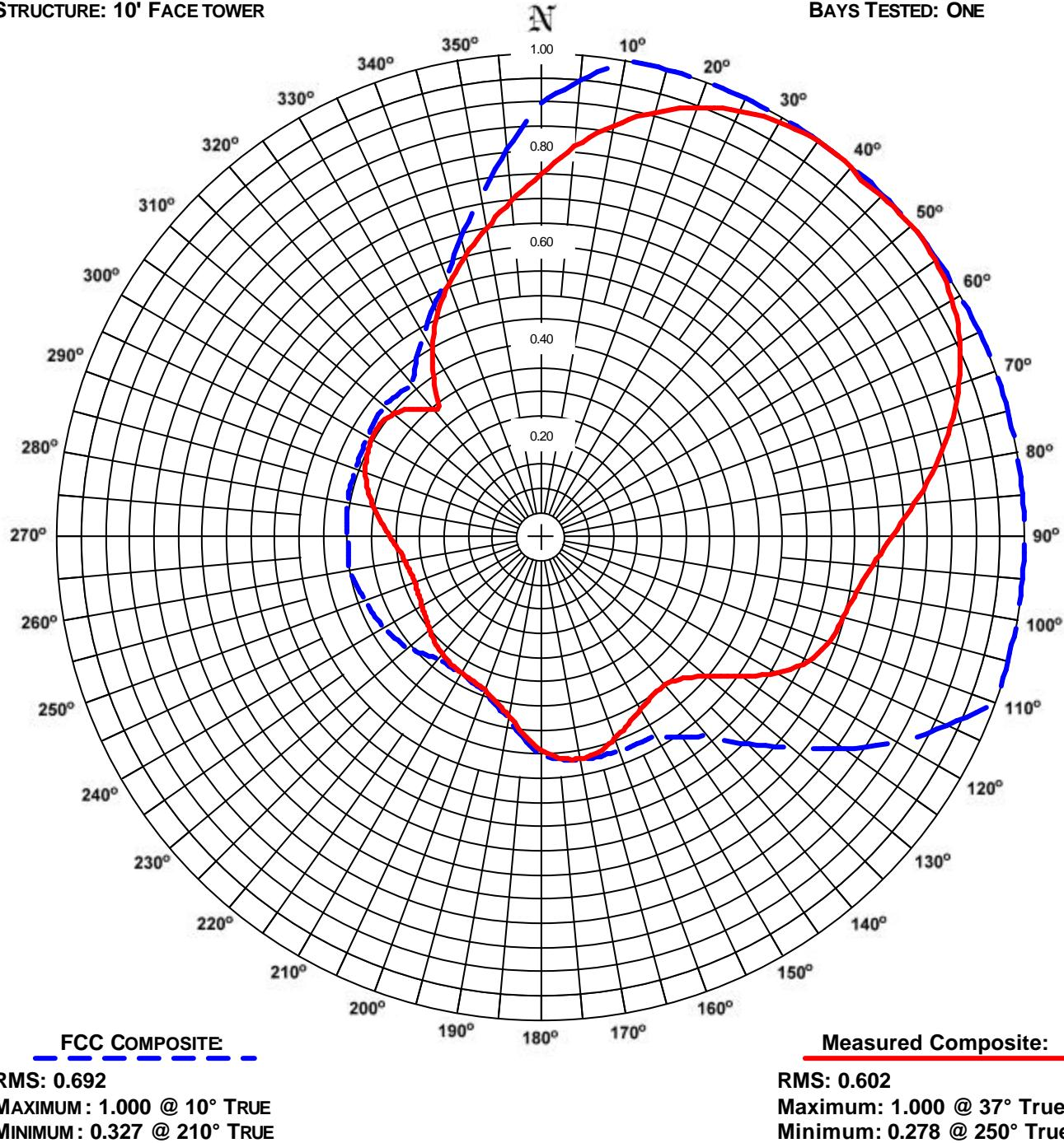
COMMENTS: COMPOSITE PATTERN: THIS PATTERN SHOWS THE MAXIMUM OF EITHER THE H OR V AZIMUTH VALUES. THIS PATTERN IS GREATER THAT 85% OF THE FCC FILED COMPOSITE PATTERN BMPED-20070827AEH.
