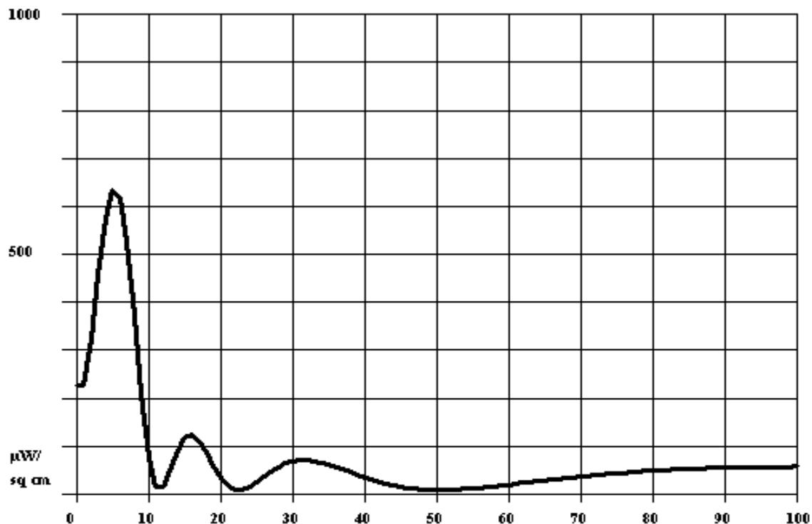
HORZ. DISTANCE FROM FM RADIATOR VS POWER DENSITY (Microwatt/Square cm)
