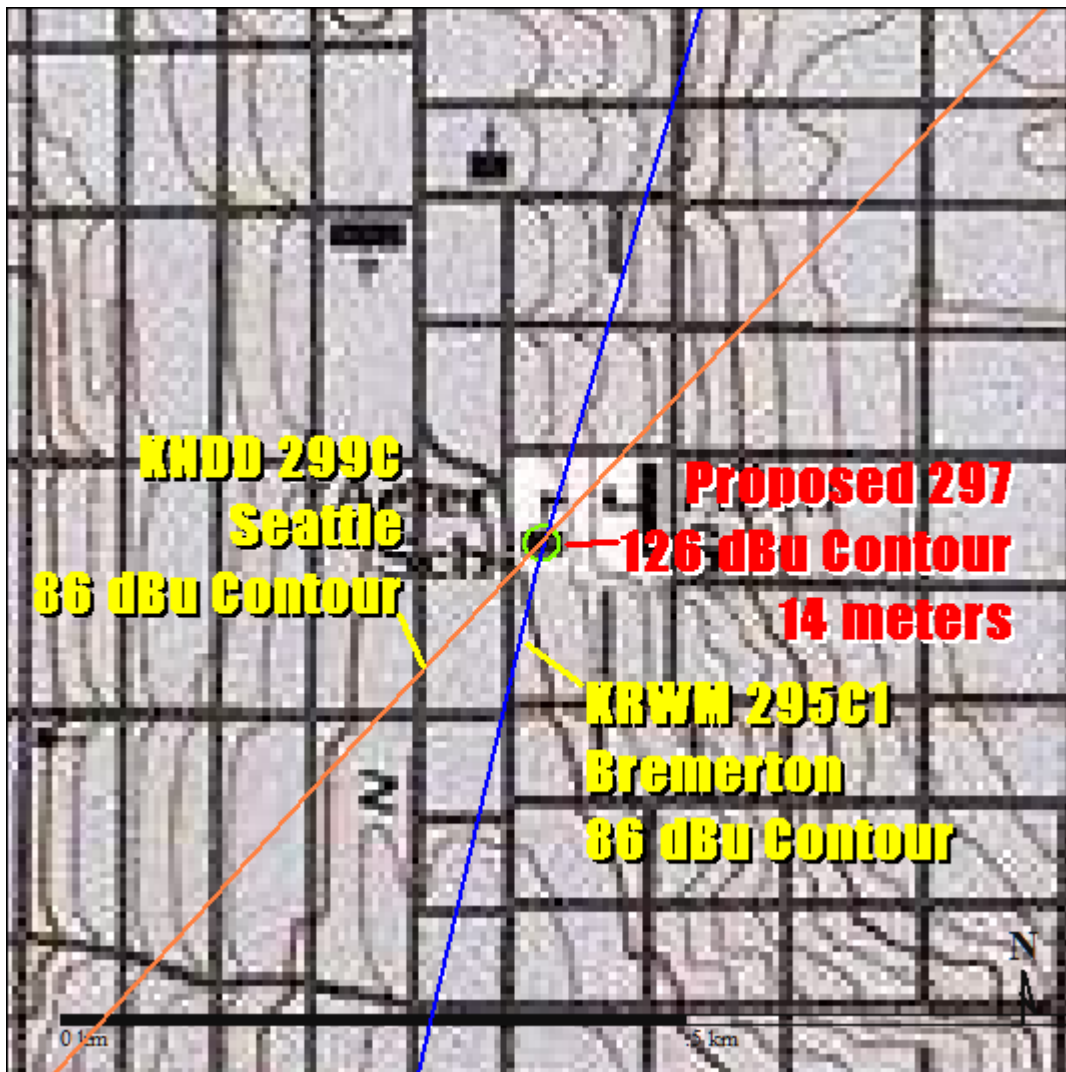
Map Showing KNDD Seattle 299C and KRWM Bremerton 295C1 86 dBu F (50,50) contours at Proposed LPFM Site and 126 dBu potential interfering contour (14 m) before suppression of downward radiation
