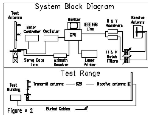
The antenna under test was operated in the transmitting mode and fed from a HP8657D signal generator. The frequency of the signal source was set at 106.7 MHz and was constantly monitored by a Rohde & Schwarz ESVD measuring receiver.
