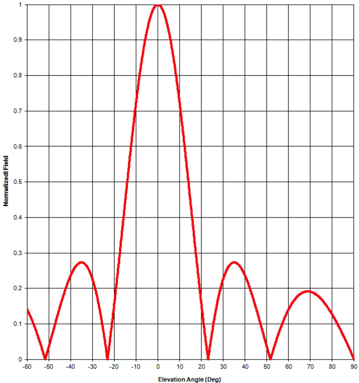
Antenna model: 6812b, 3-bay full-wave-spaced
