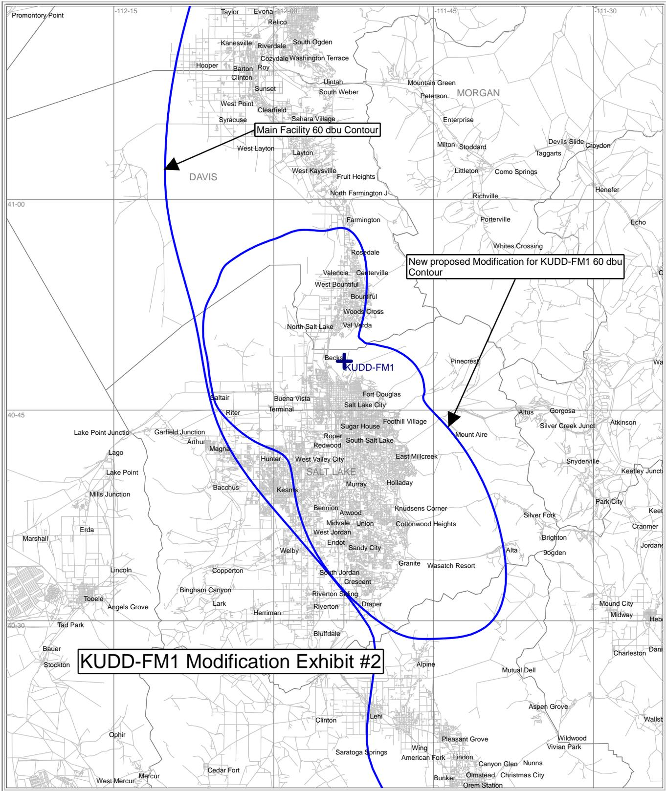
Proposed modifications for facility 2100 watts 130 degrees
