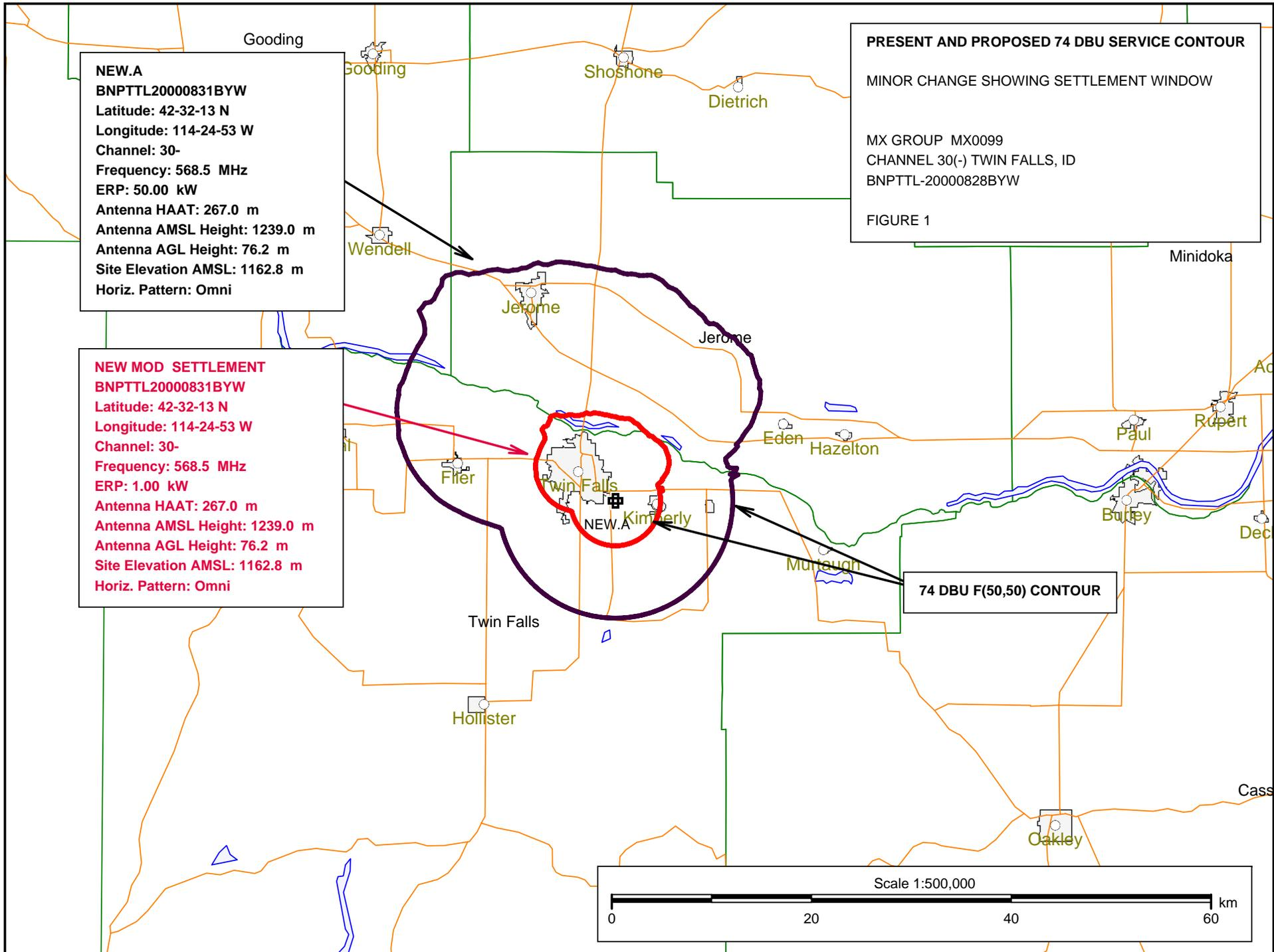
FIGURE 2 - OET BULLETIN NO. 69 INTERFERENCE STUDY RESULTS FOR MX GROUP MX0099
