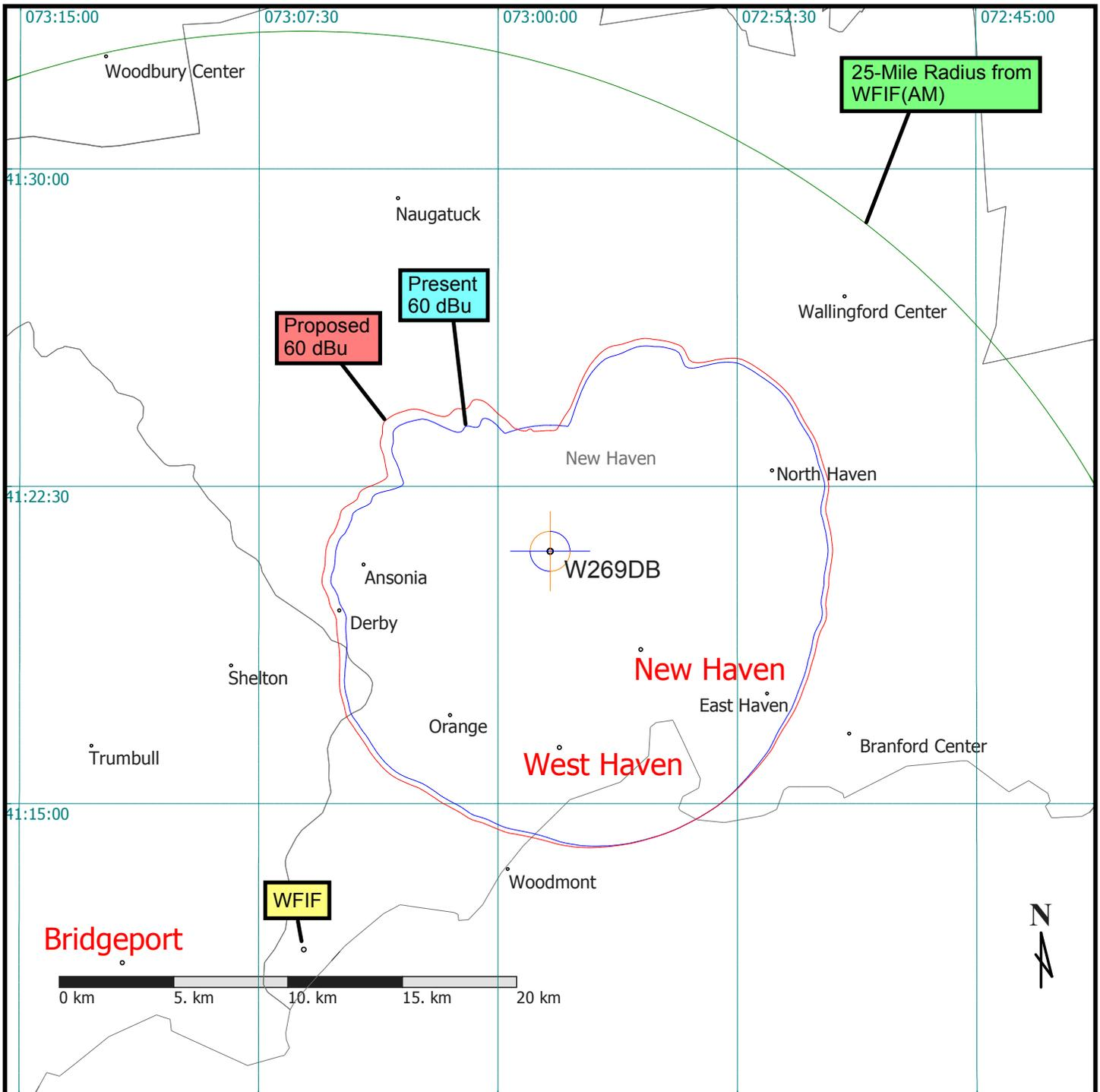
Figure 2 -- Co-Channel and First-Adjacent Interference Contours
