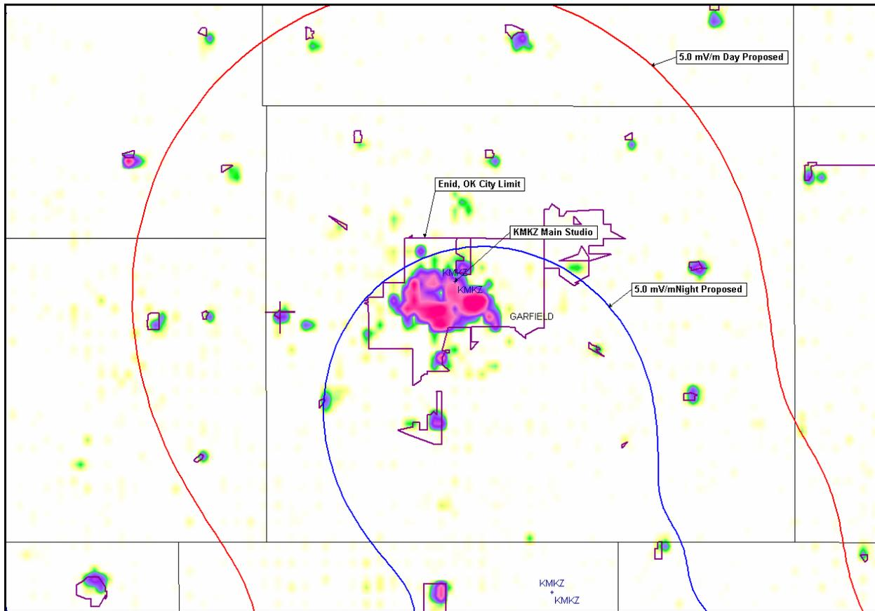
The KMKZ main studio location is located within both the 5.0 mV/m proposed day contour and the 5.0 mV/m proposed night contour, in accordance with §73.1125 of the Commission's Rules.
