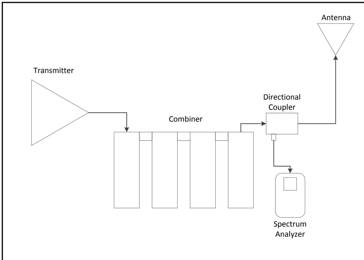
Intermodulation Frequency Measurement Configuration
