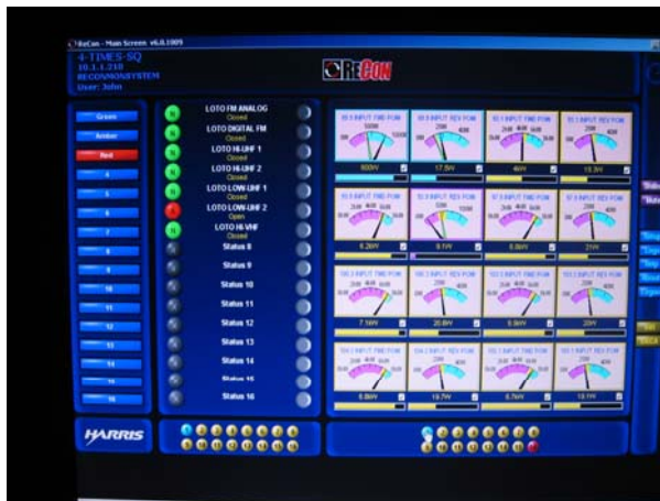
Figure 12. CRT display of the Harris RECON™ system used for continuous monitoring of the status of each transmitter at the 4TS facility. Trip points may be set to cause activation of alarms based on transmitter power levels.
