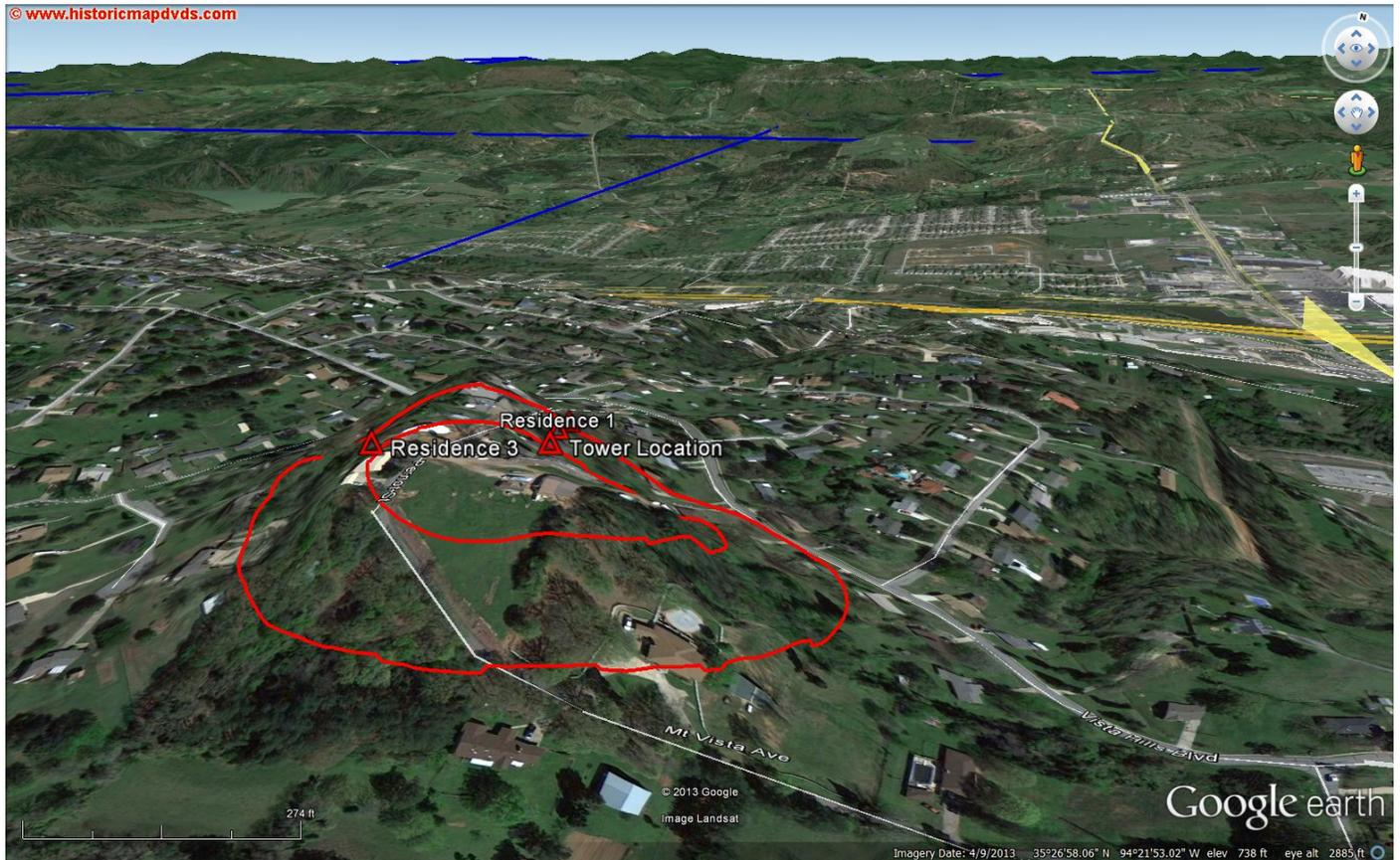
This second image exaggerates the terrain in the vicinity of the tower to definitively illustrate that it does site on a ridge. From this image it can be inferred that the terrain changes sufficiently that the interference zone will overshoot nearly all of the structures lying between the two rings comprising the interference zone. Residence 1 and Residence 2 to the north of the tower site are of initial interest.
