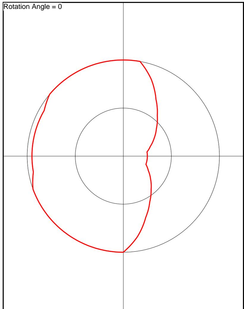
The KMTT Auxiliary antenna is a Shively panel antenna consisting of 2 panels at 6 levels. This antenna is used by seven other FM stations.
