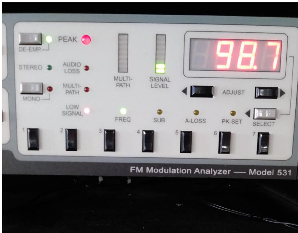
This picture shows DEV/Modulation is peaking at 89% which is the same as the primary station being received at the time of reading.
