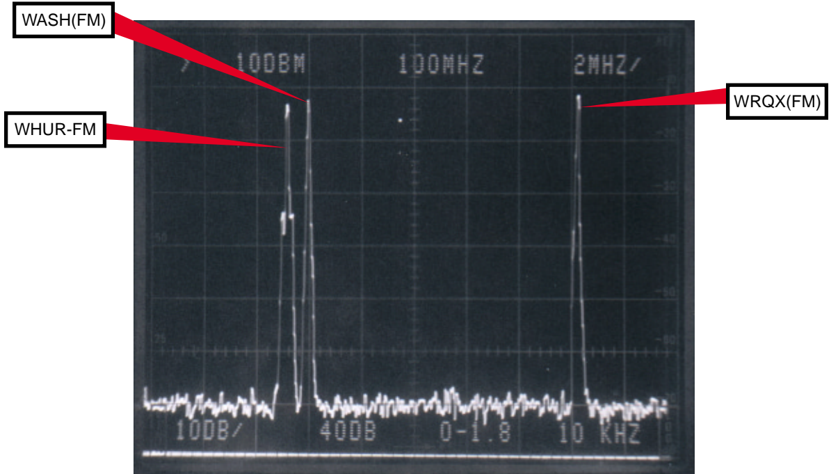
Plot 7 WRQX(FM), WHUR-FM and WASH(FM) at combiner output
