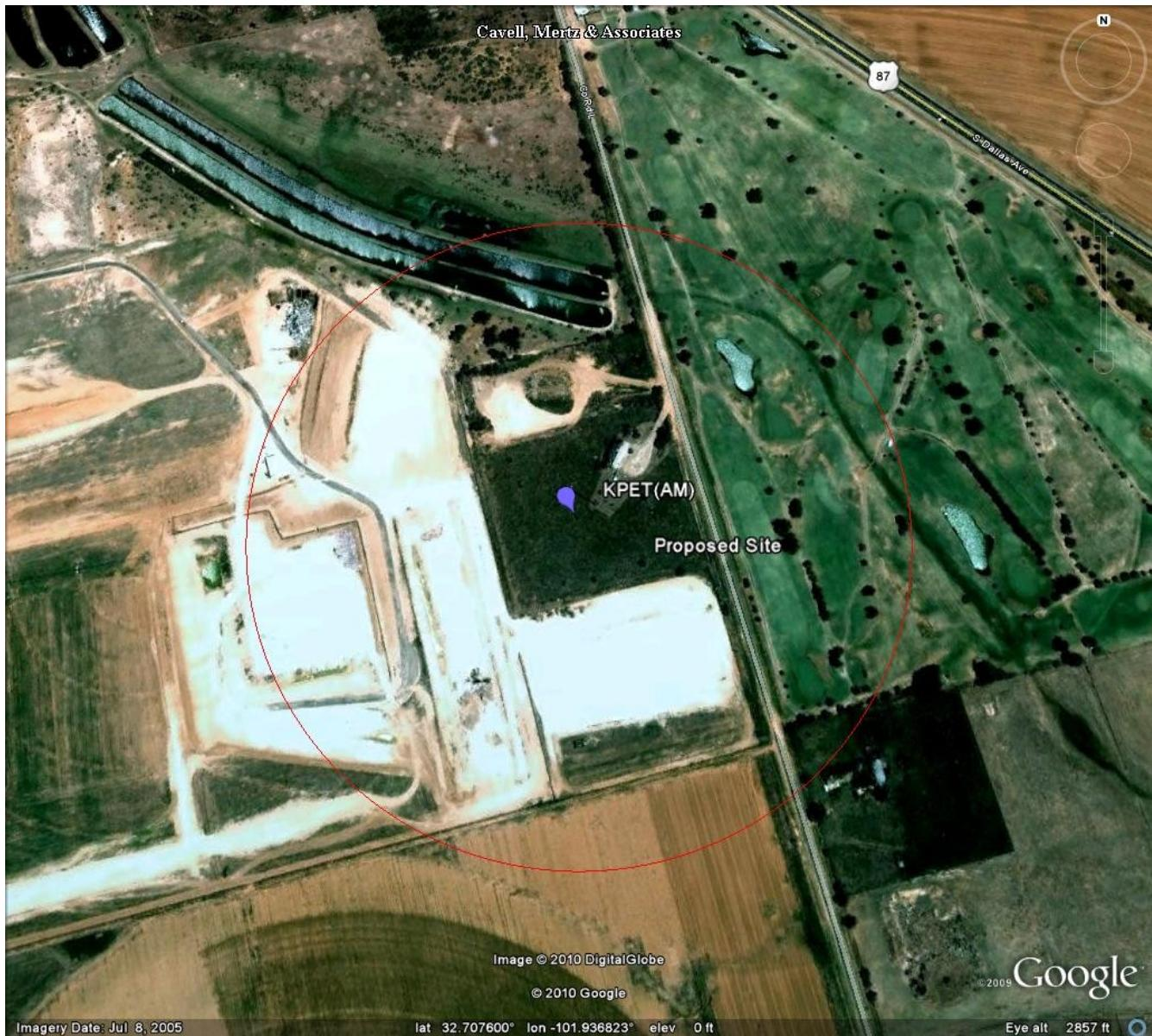
The red circle shows a 300 meter radius (Free Space distance to contour predicted to cause interference to KXTC). Actual distance is less as this ignored antenna vertical pattern, and the fact that the antenna is elevated 80 meters above ground. This worst case falls short of the one house on this page (to south east).
