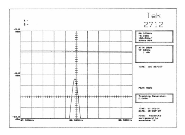
**Note:** Upper trace is output of tracking generator with attentation pads only. Lower trace is with tunable bandpass cavity inserted between pads. Measured insertion loss is therefore 2.6 db.
