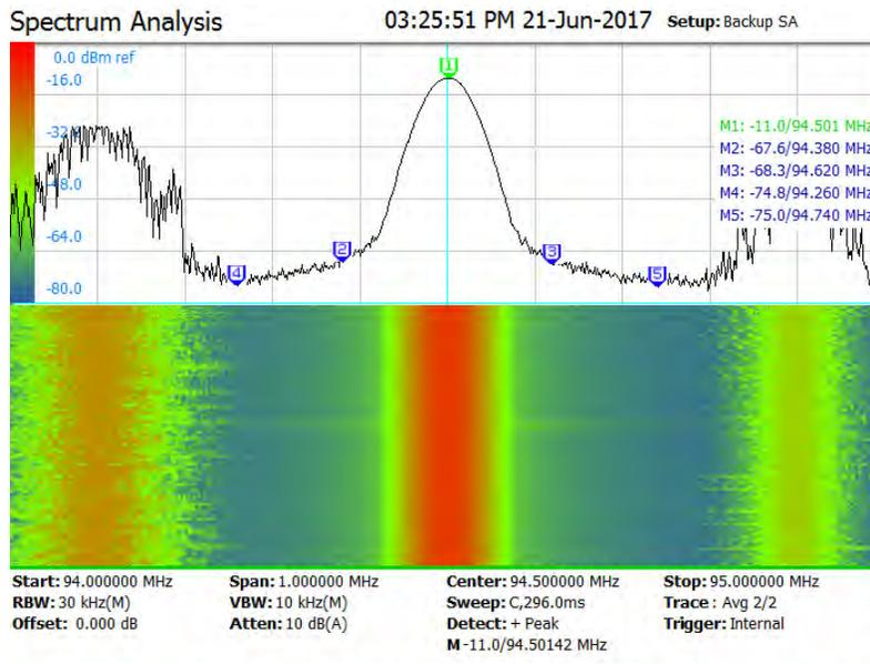
4. Readings of 240, and 600 kHz off Center Frequency 94.500 MHz
