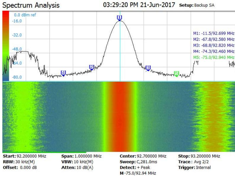
2. Readings of 240, and 600 kHz off Center Frequency 92.700 MHz
