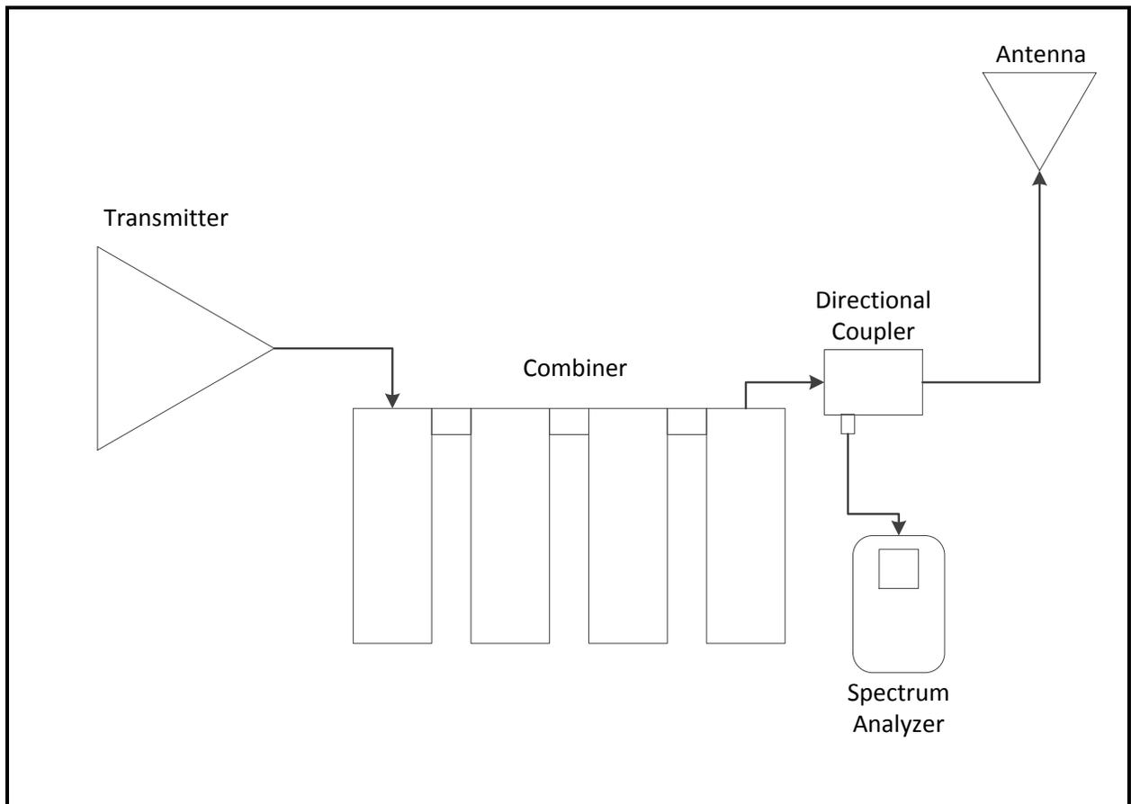
Intermodulation Frequency Measurement Configuration
