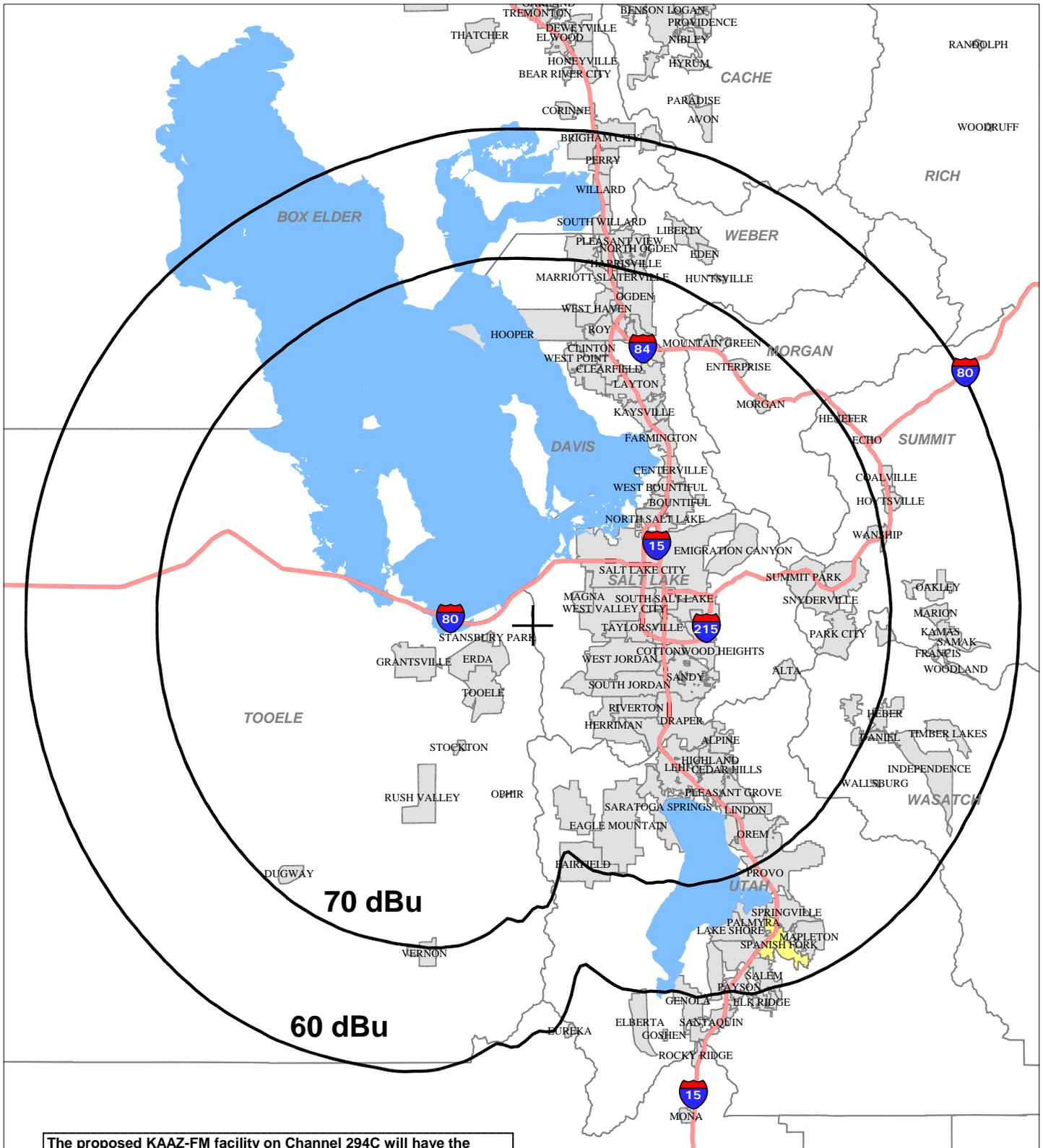
The proposed KAAZ-FM facility on Channel 294C will have the same technical parameters (site, height, and ERP) as the licensed KAAZ-FM facility on Channel 293C. It was previously demonstrated in BMPH-20011206AAT that this facility would provide at least 70 dBu service to 100% of Spanish Fork.
