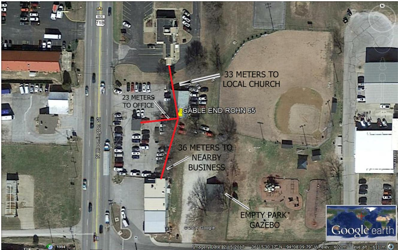
Radiation center at 19 meters above ground level
