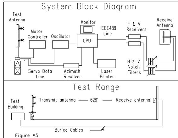
The antenna under test was operated in the transmitting mode and fed from a HP8657D signal generator. The frequency of the signal source was set at 107.5 MHz and was constantly monitored by a Rohde & Schwarz ESVD measuring receiver.
