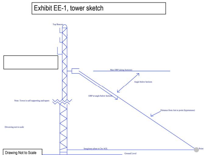
$\text{DistToPoint} = \text{Antenna Rad Center in meters AGL} / (\text{Cos}(90^\circ - \text{Angle}))$
