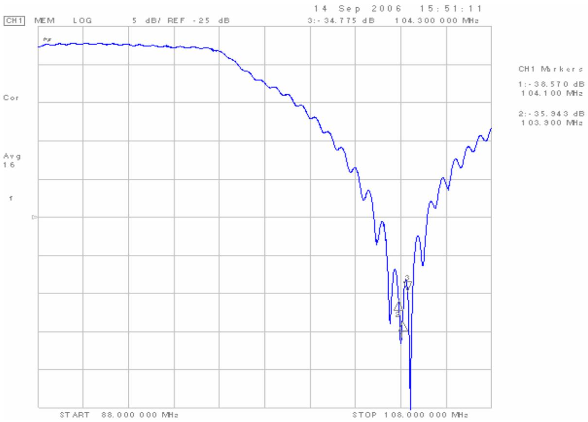
20 MHz Span Return Loss Plot
