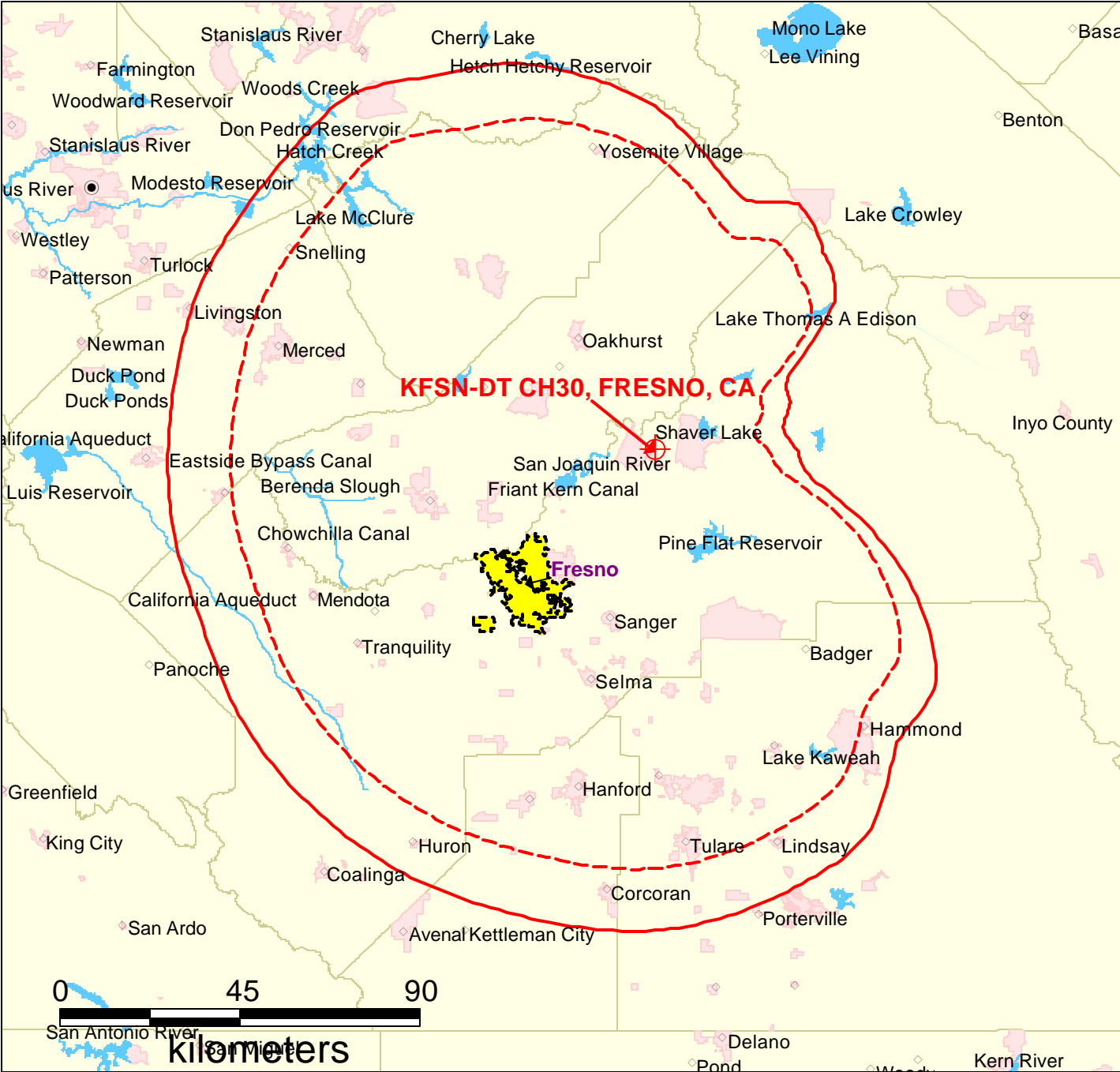
PREDICTED COVERAGE CONTOURS KFSN-DT Ch 30, Fresno, CA 260 kW, 625 mHAAT 1458 mRCAMSL, ATW30HAZ-CX-30H D-ANT
