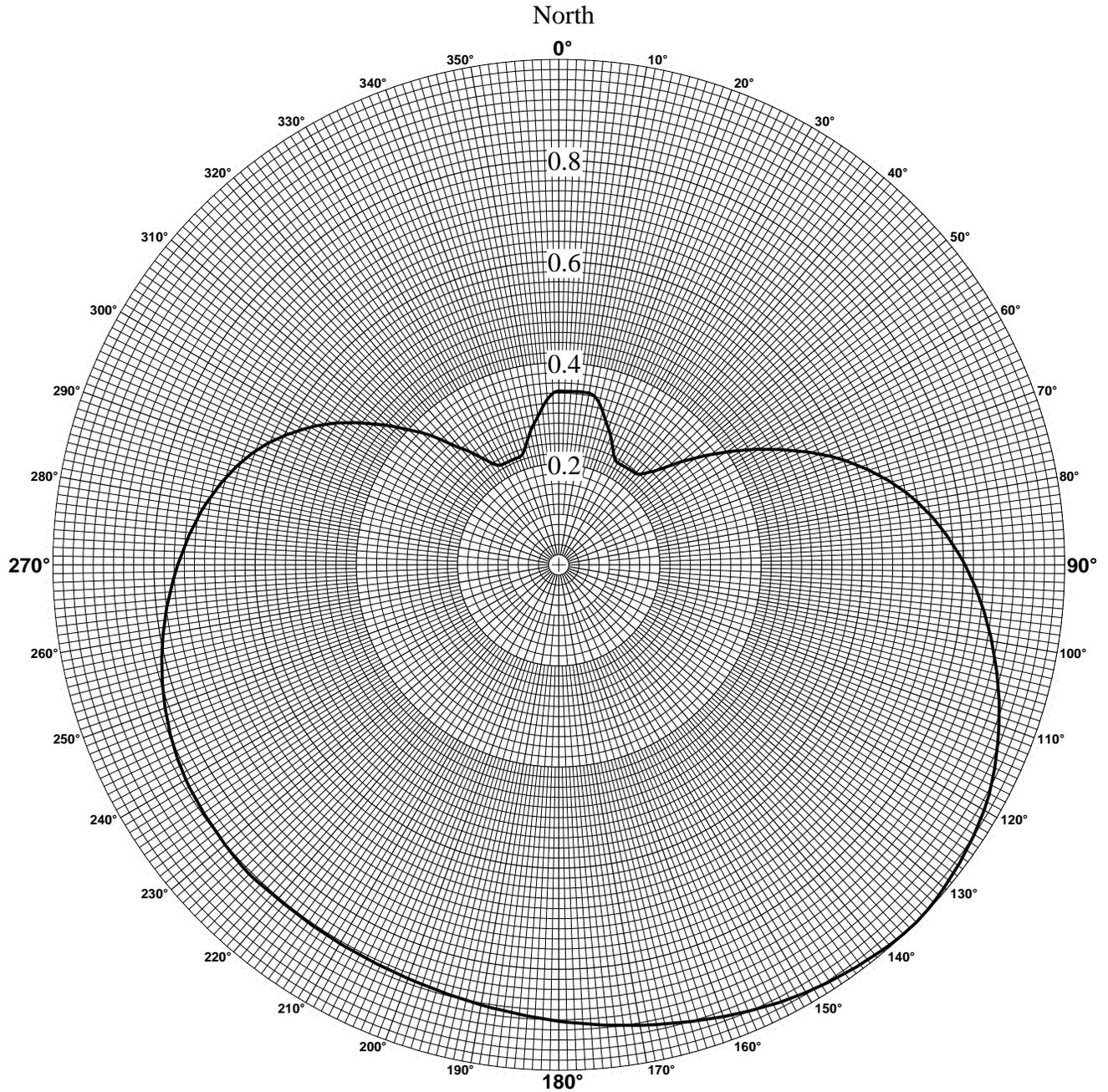
Note: Pattern is based on manufacturer's supplied data and reflects use of electrical and mechanical beam tilts.
