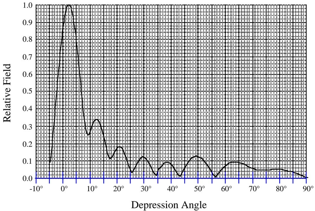
Note: Pattern is based on manufacturer's supplied data. Indicated electrical beam tilt of 1.75° applies at azimuths of 125°T and 305°T.
