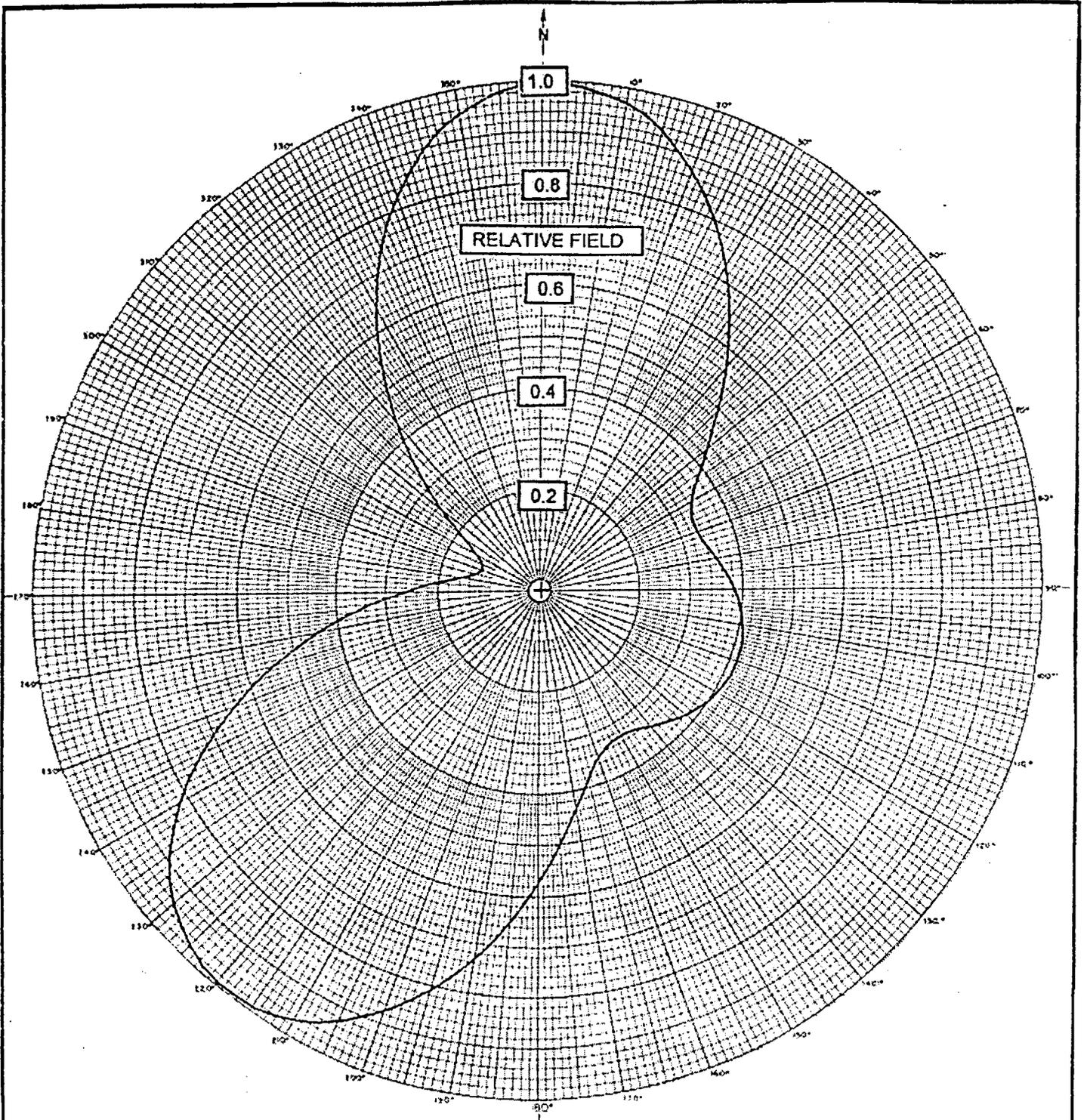
PROPOSED BEARING OF ANTENNA: N 290° E
