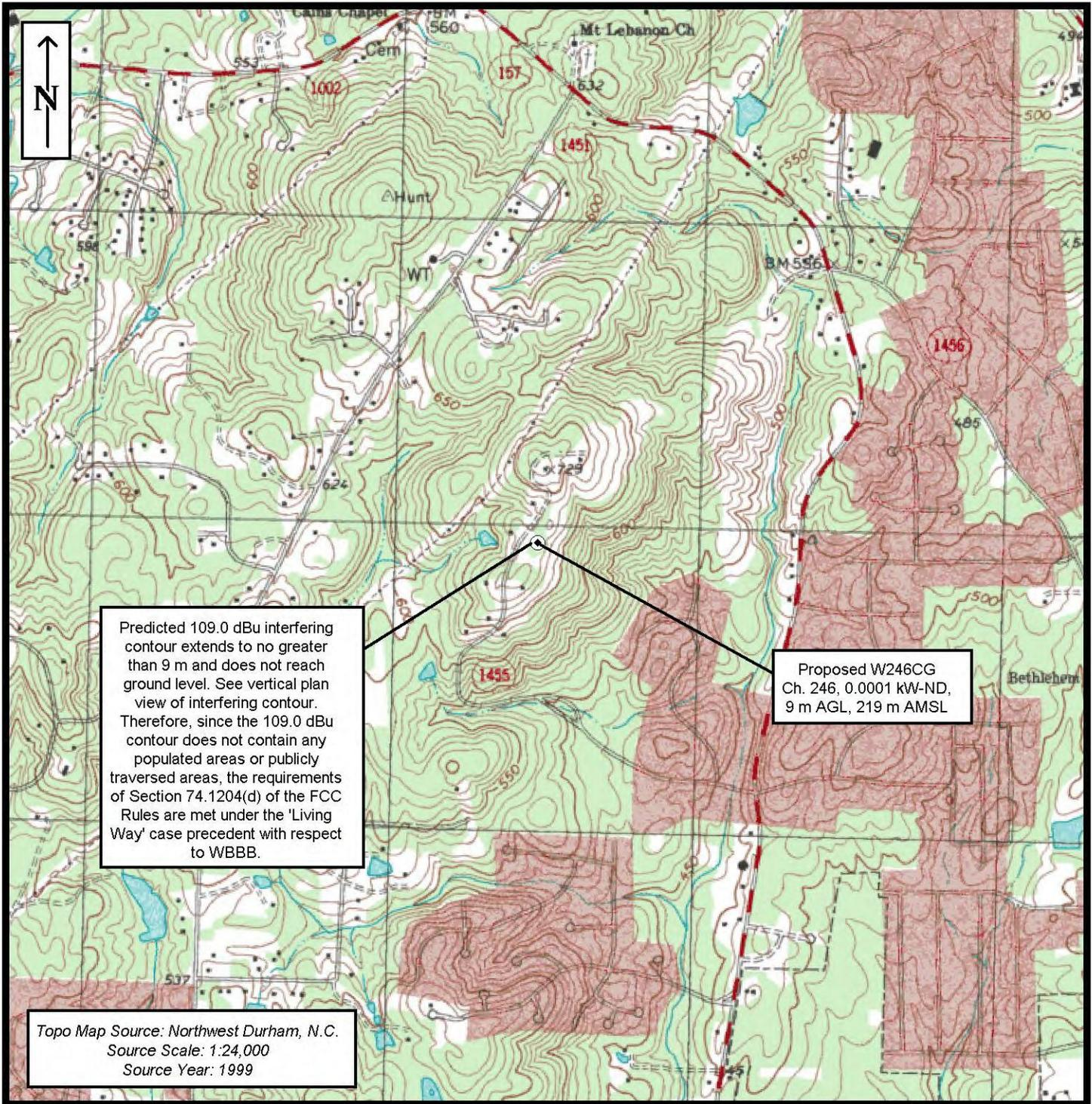
Predicted 109.0 dBu interfering contour extends to no greater than 9 m and does not reach ground level. See vertical plan view of interfering contour. Therefore, since the 109.0 dBu contour does not contain any populated areas or publicly traversed areas, the requirements of Section 74.1204(d) of the FCC Rules are met under the 'Living Way' case precedent with respect to WBBB.
