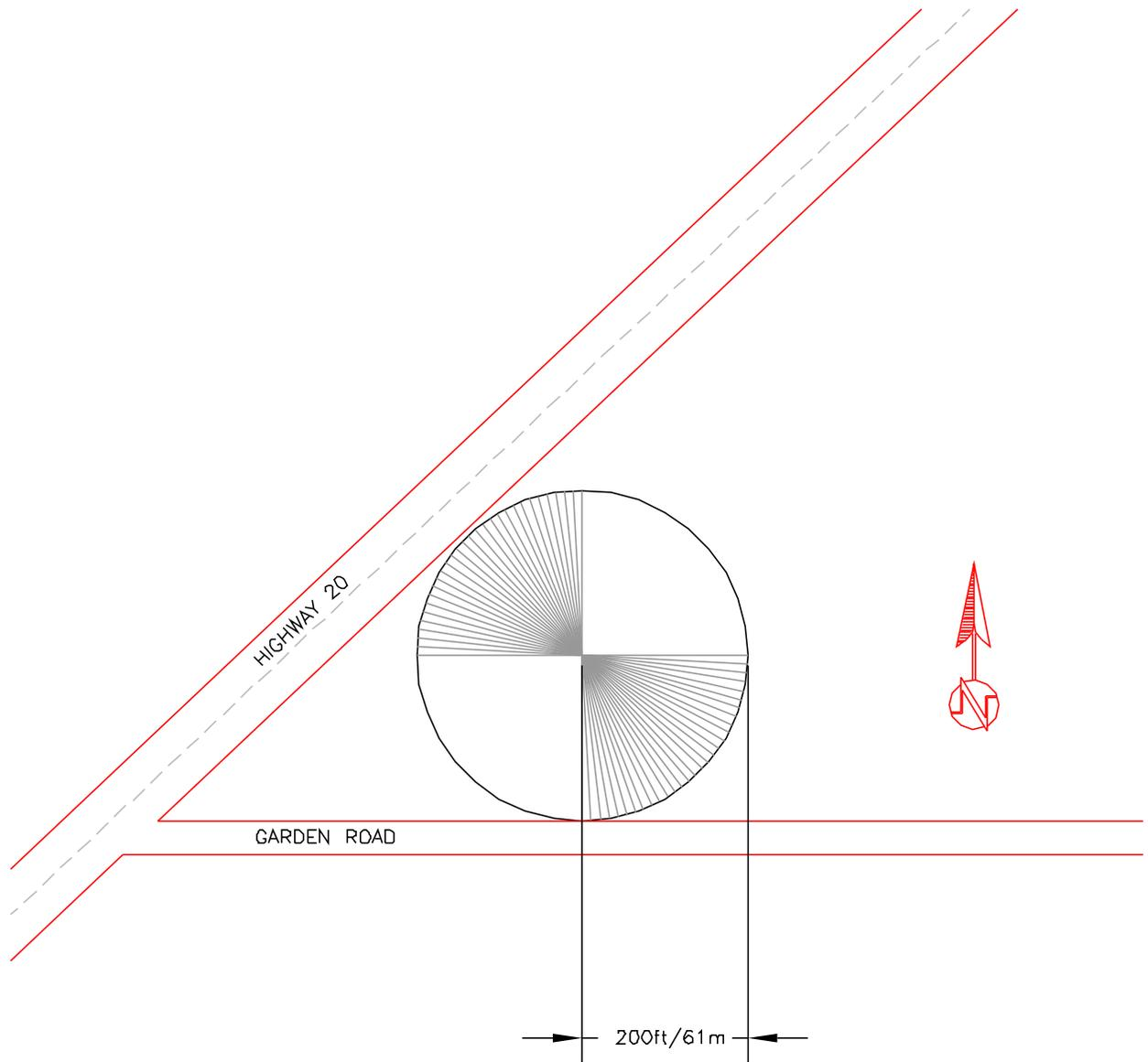
GROUND SYSTEM CONSISTS OF 120 RADIALS SPACED EVERY 3' ABOUT EACH TOWER
