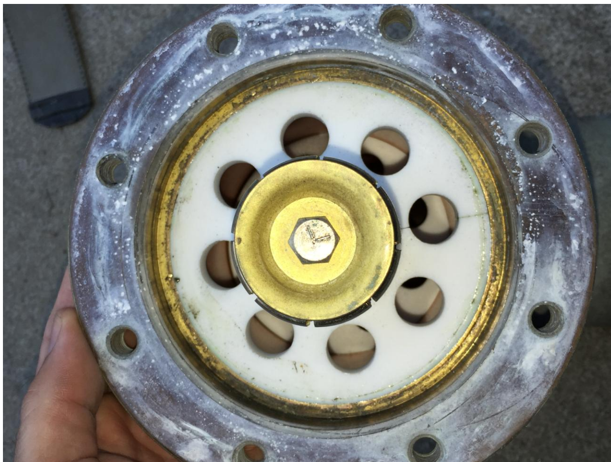
Unibolt elbow with contaminated RF lip
