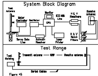
The measurements were performed by rotating the test antenna in a counter-clockwise direction and plotting the received signal on polar coordinated graph paper in a clockwise direction. Both horizontal and vertical components were recorded separately.
